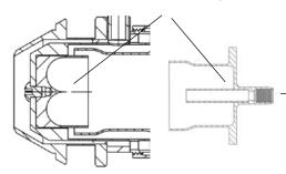
Unscrew nozzle nose, remove collector and unscrew tip.
